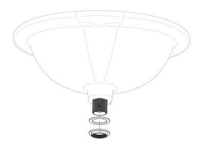
3. Fit waste trap to waste grate, following the trap installation guide
